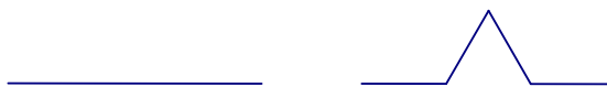
FIGURE 16. Edge and its replacement in the iterative construction of the Koch snowflake
